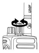
Once the required zone is displayed (if you have multiple zones in your radio), turn the programmed Channel Selector Knob to select the call type.
